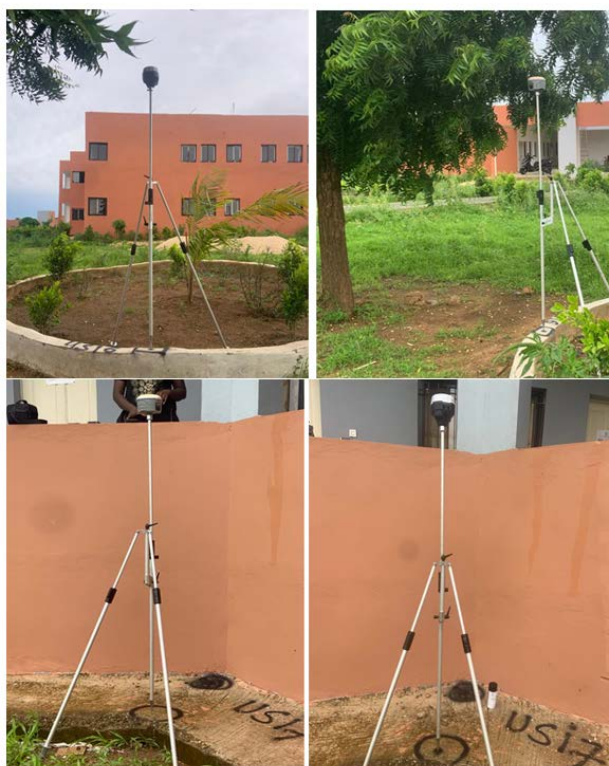
Figure 6. Observation of US16 and US17 points in NRTK with Emlid RS2+ and CHC i50 receivers.
