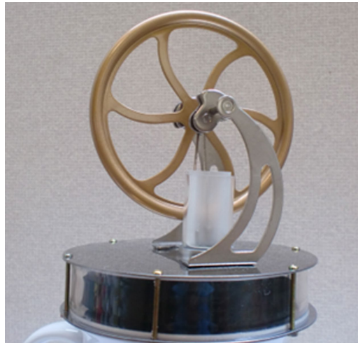
Figure 2. A low temperature Stirling engine (LTSE) works with heat flows (entropy flows) in NISs [18].
