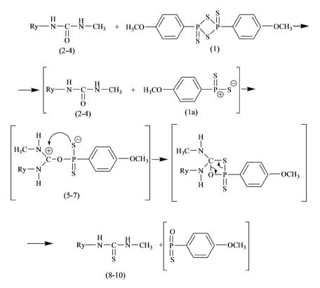
**Figure 2.** The thionization mechanism for glycosylurea (where Ry = xylose, glucose, and galactose).
