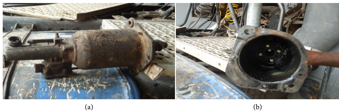
Figure 1. Typical actuator chamber of a heavy duty vehicle. (a) Longitudinal view (b) Cross-sectional view.
