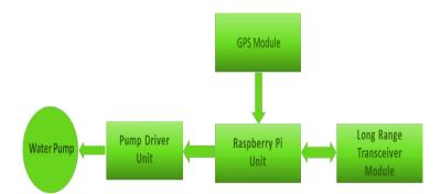
Figure 11. Actuator node architecture.
