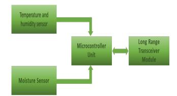
Figure 10. Sensor node architecture.
