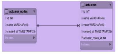
**Figure 12.** Actuator database design model.
