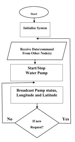
Figure 9. Actuator Node flowchart.
