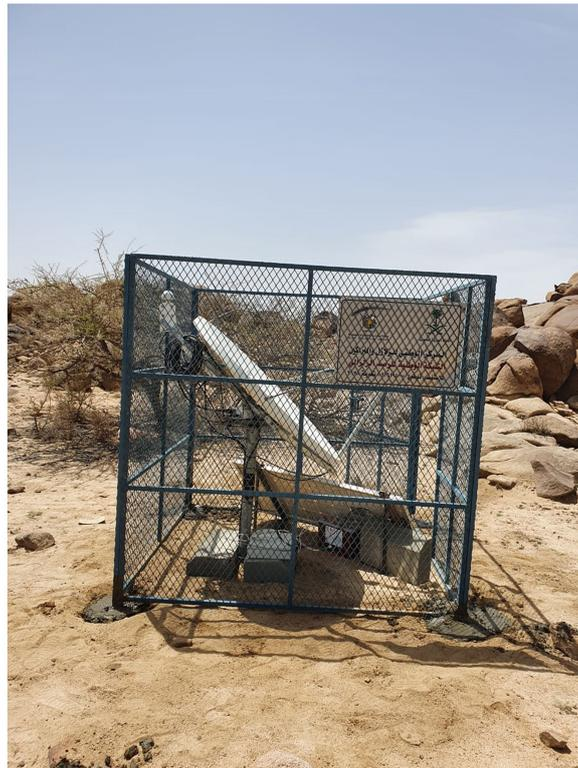
**Figure 5.** A photo of a complete seismic monitoring station (weak motion station) that was established in the epicenter area of the Khamis Mushait earthquake, on the edge of the lake and ~7 km to the east of the Tandaha dam.
