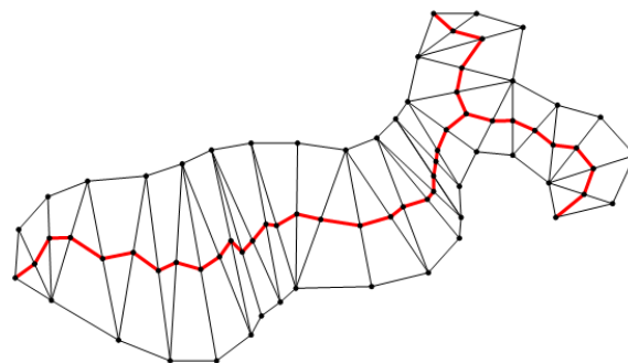
Figure 17. The center axis acquired by gravity method (2D view).
