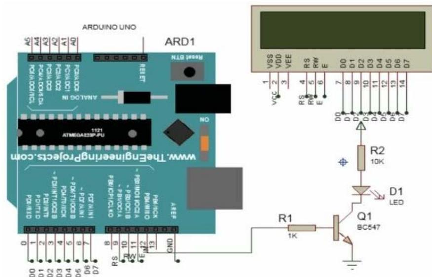
**Figure 5.** Li-Fi transmitter block.
