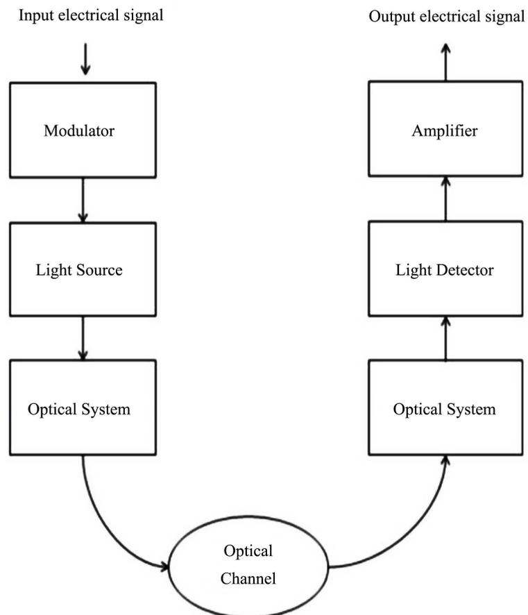
**Figure 3.** Block diagram of VLC system.
