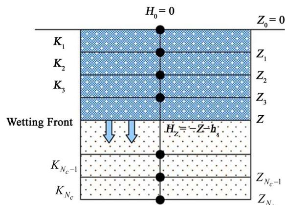
**Figure 3.** Infiltration into a layered soil profile under an initially ponded condition [5].
