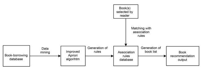
Figure 3. Structure diagram of personalized information recommendation submodule.
