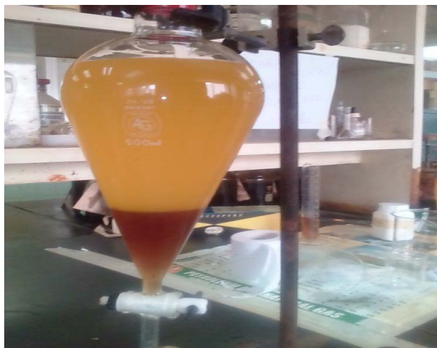
Figure 1. Synthesized bio-glycerol (lower layer) and methyl esters (upper layer).
