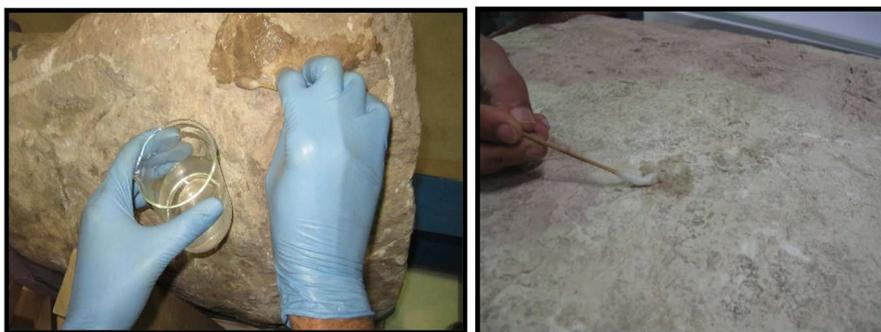
**Figure 23.** Part of the chemical cleaning of the stone objects.
