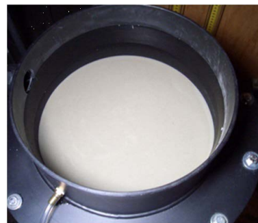
Figure 4. Photographic top view of sample after pluviation of soil material A1 under de-aired water.
