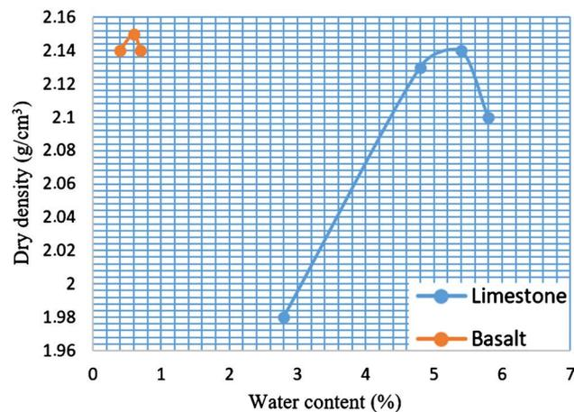
**Figure 4.** Compaction curves of materials studied.
