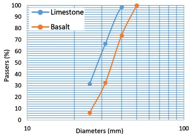
**Figure 3.** Grain size curves of aggregates of Bandia Limestone and Diack Basalt.
