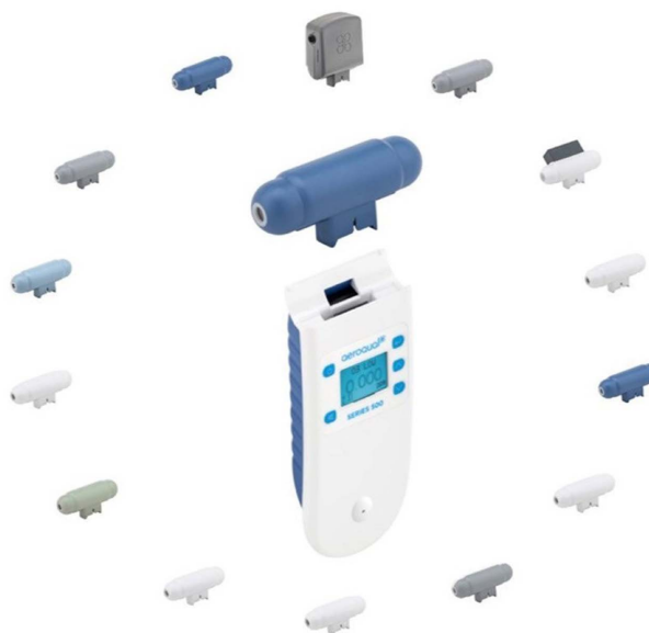
Figure 1. Aeroqual handled air quality monitor with sensors. (PM 2.5 , PM 10 , CH 4 , CO, Cl 2 , NH 3 , SO 2 , NO 2 , CO 2 ).
