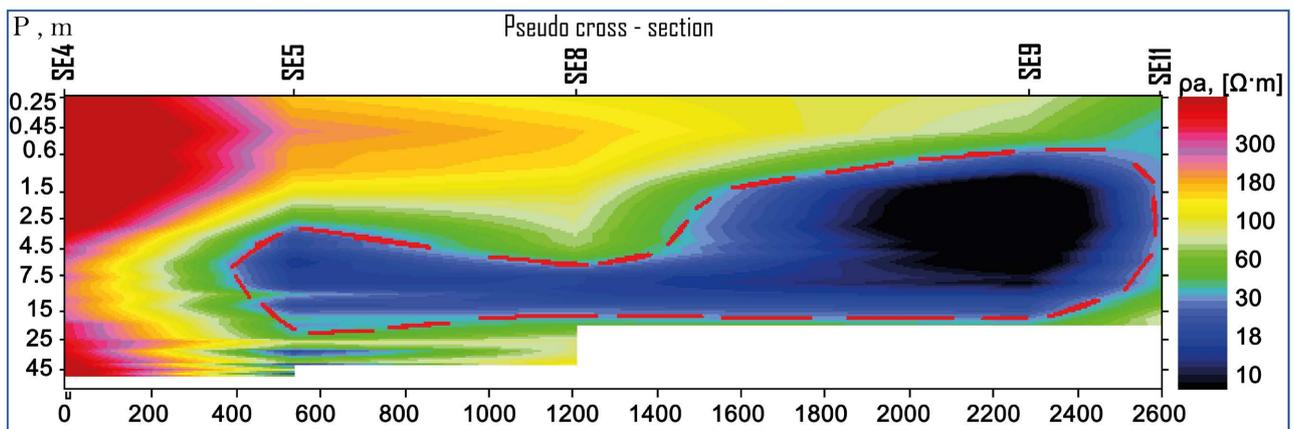
Figure 9. Geoelectrical longitudinal section of the Akouédo landfill.
