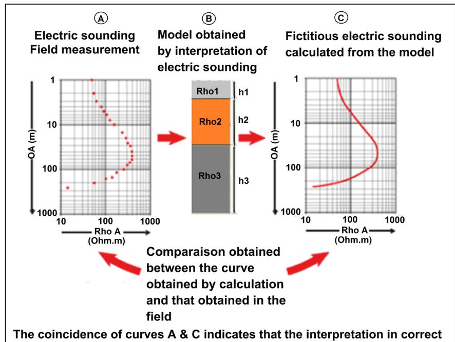
**Figure 4.** Model for modeling and inversion of electrical sounding curves (Kouakou et al., 2012).
