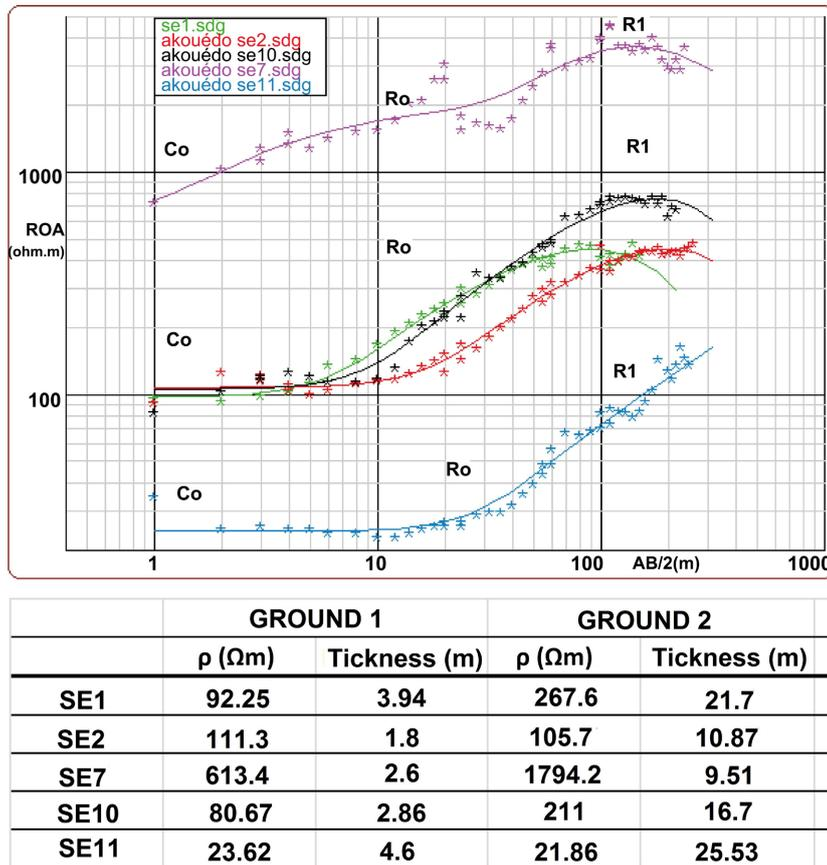
Figure 6. Family sampling curves 1. -: Indefinite thickness.
