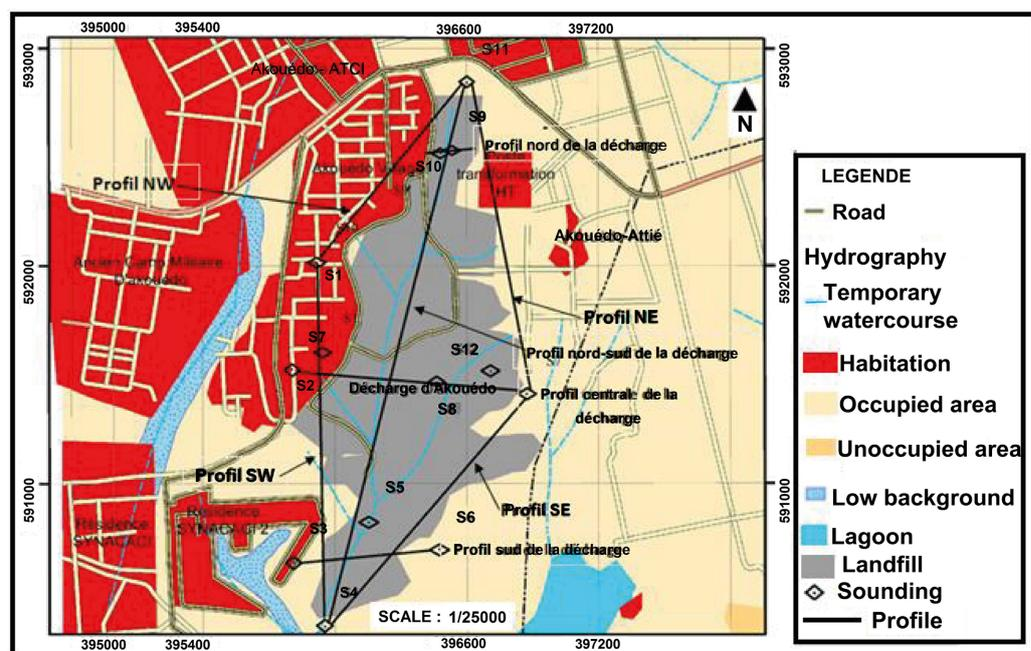
Figure 3. Positioning plan for electrical sounding waypoints.
