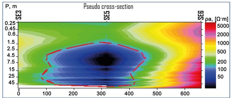
**Figure 10.** Geoelectrical cross section of the Akouédo landfill.
