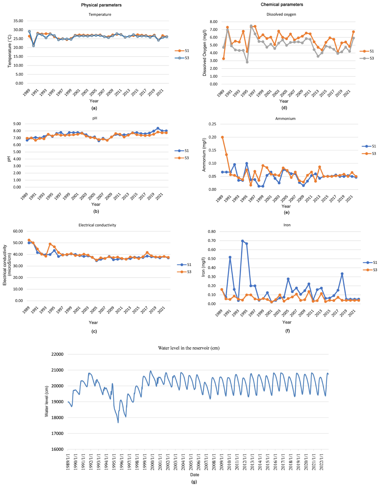
Figure 4. (a) Annual temperature variation in stations; (b) Annual pH variation in stations; (c) Annual electrical conductivity variation in stations; (d) Annual dissolved oxygen variation in stations; (e) Annual ammonium content variation in stations; (f) Annual iron content variation in stations; (g) Variation of the water level in the reservoir from 1989 to 2022.
