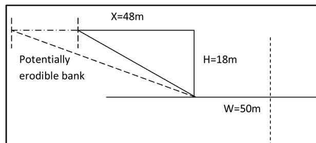
**Figure 8.** Dimensions of a section of the channel.
