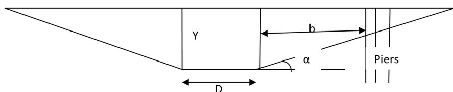
**Figure 10.** Schematics for assessing area of influence of sub-aqueous borrow pit.  $\alpha$  = angle of repose.  $D$  = diameter of borrow pit.
