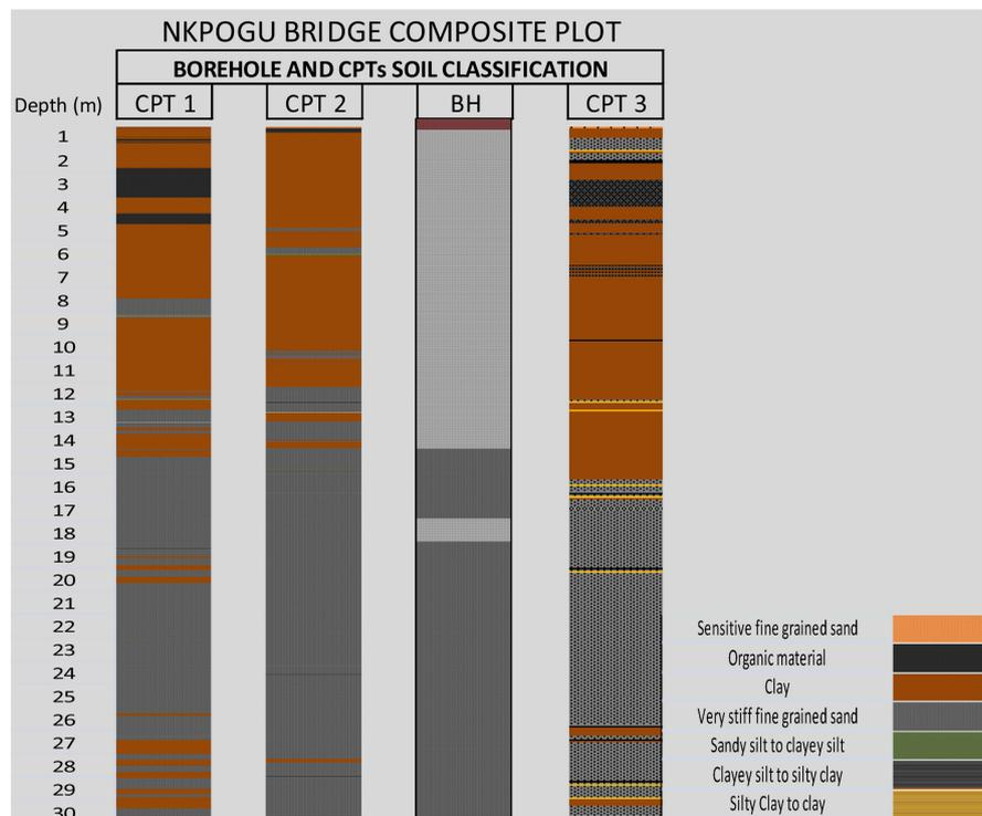
**Figure 7.** Lithostratigraphy composed of borehole log and CPT based SBT classification.
