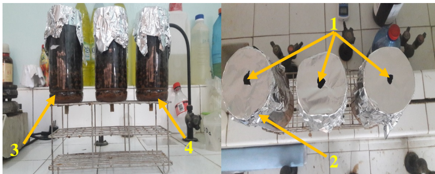
Figure 1. Batch assay on substrate of coated “jujube” seeds as medium filtering and fixation of bacteria for removal of Fe (II); 1—natural ventilation holes, 2—aluminum foil used as cover, 3—phase clear and hazy phase separation, 4—sludge.
