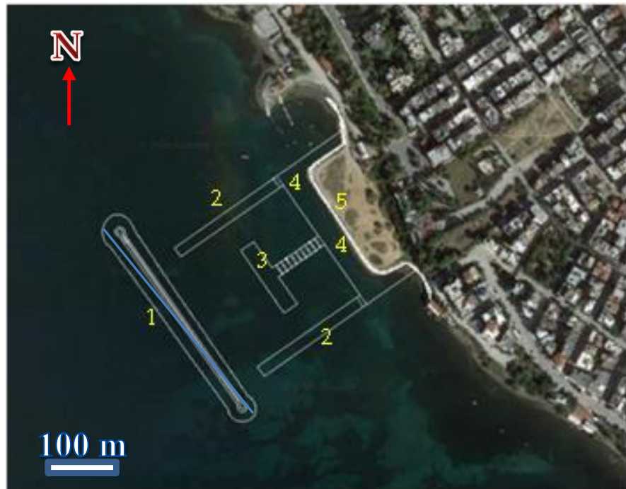
Figure 2. The basic design of the harbor with the basic structural elements noted with numbers as follows: 1 shows the breakwater detached and parallel to the coastline, number 2 shows the two leeward external moles-groins with total length 155 m, number 3 shows the inner mole-pier of T shape in the middle of the basin, number 4 shows the seawalls and all the operational surfaces behind the walls and number 5 shows the land zone.
