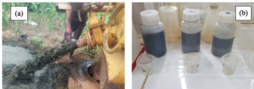
Figure 1. Collection of sludge on the landfill site and presentation of the 3 samples in the laboratory.
