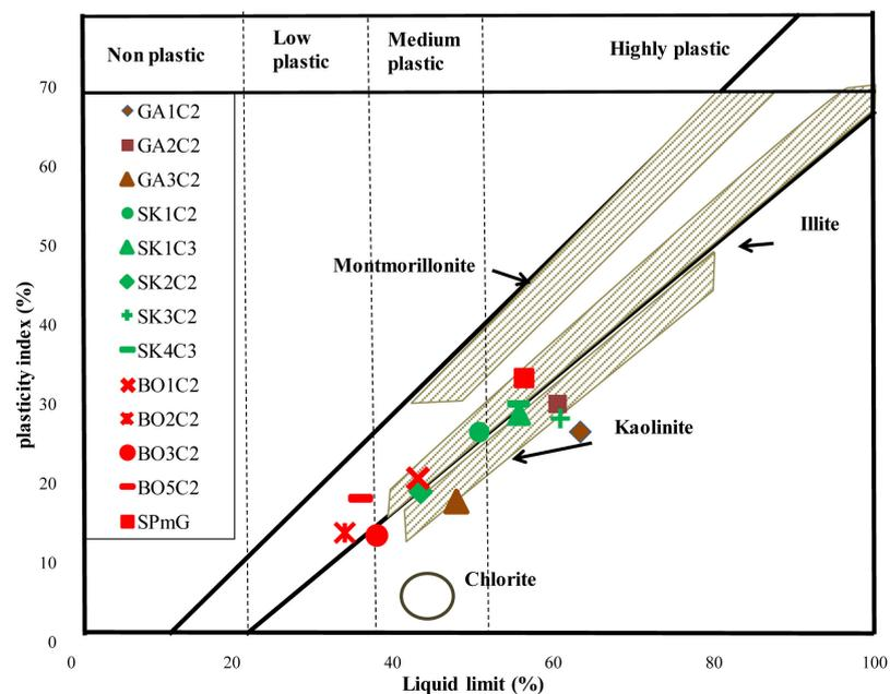
Figure 3. Casagrand's plasticity chart (Holtz & Kovacs, 1981) showing representative clay material samples.
