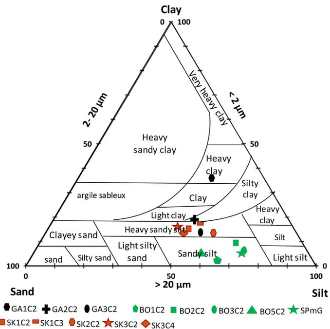
**Figure 5.** Ternary diagram of the studied clay materials samples according to Richer de Forges et al. (2008).
