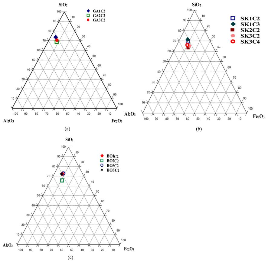
**Figure 4.** Geochemical composition of the studied soils in SiO<sub>2</sub>-Al<sub>2</sub>O<sub>3</sub>-Fe<sub>2</sub>O<sub>3</sub> diagram, (a) Gaschiga; (b) Sekandé and (c) Boulgou.
