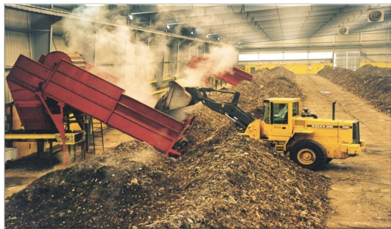
Figure 2. Aerobic windrow system at greensite composting plant.
