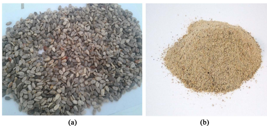
Figure 1. Whole seeds (a) and particles with particle size less than 6000 µm (b).
