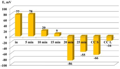
**Figure 4.** Variation of pH values and redox potential (E, mV) when electroactivating undiluted RBY (C1).  $j = 20 \text{ mA/cm}^2$ ; CC S—Cathode cell content (foam phase); CC L—Cathode cell content (liquid phase).
