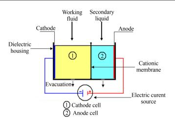
Figure 2. Scheme of the EDP-0.5 diaphragm electrolyzer.
