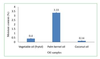
Figure 1. Moisture content of different oil samples.
