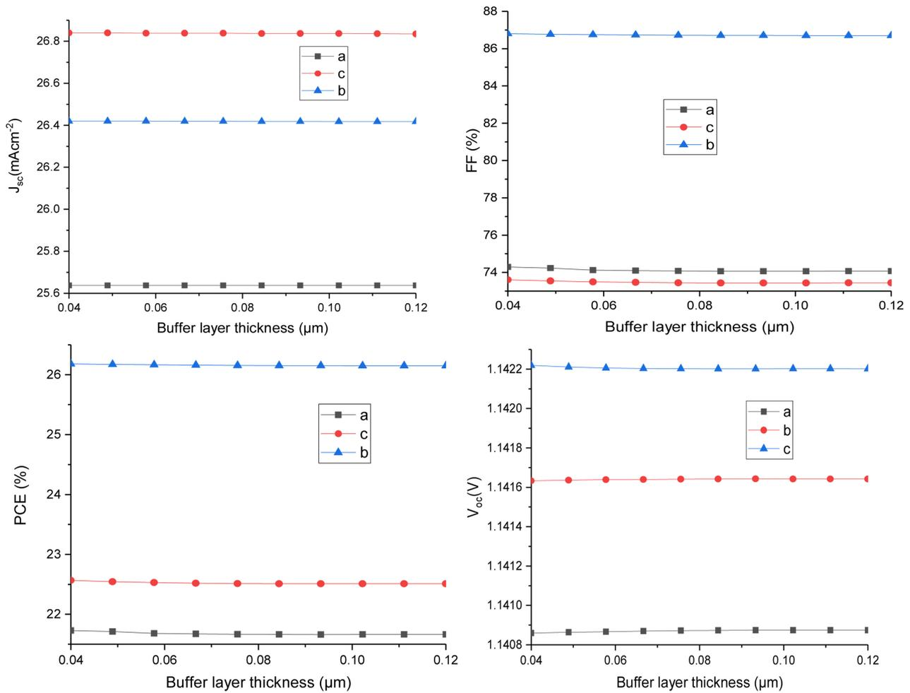
**Figure 4.** The variation of buffer layer thickness and corresponding change in electrical parameters of solar cell (a = 0.6  $\mu\text{m}$ , c = 1  $\mu\text{m}$ , b = 0.8).
