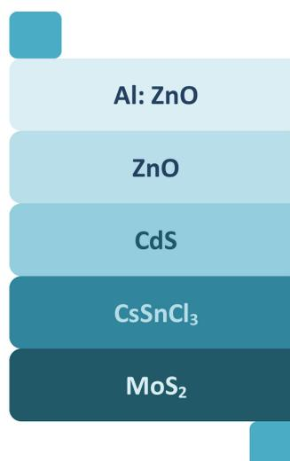
**Figure 1.** The suggested perovskite solar cell.
