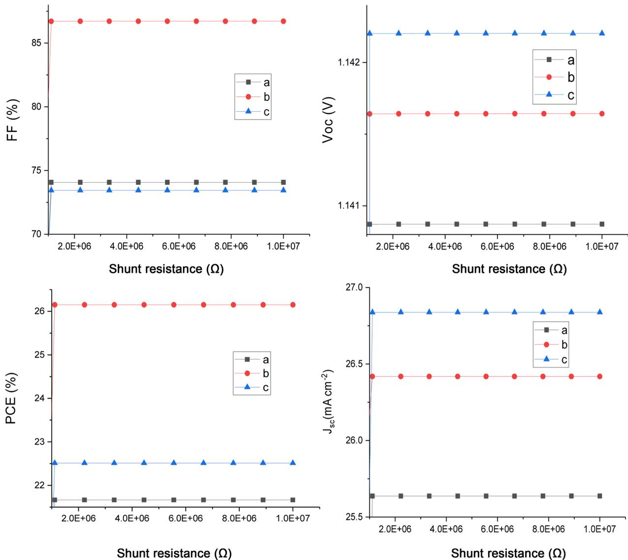
**Figure 3.** Effect of shunt resistance on various electrical characteristics ( $a = 0.6 \mu\text{m}$ ,  $c = 1 \mu\text{m}$ ,  $b = 0.8$ ).
