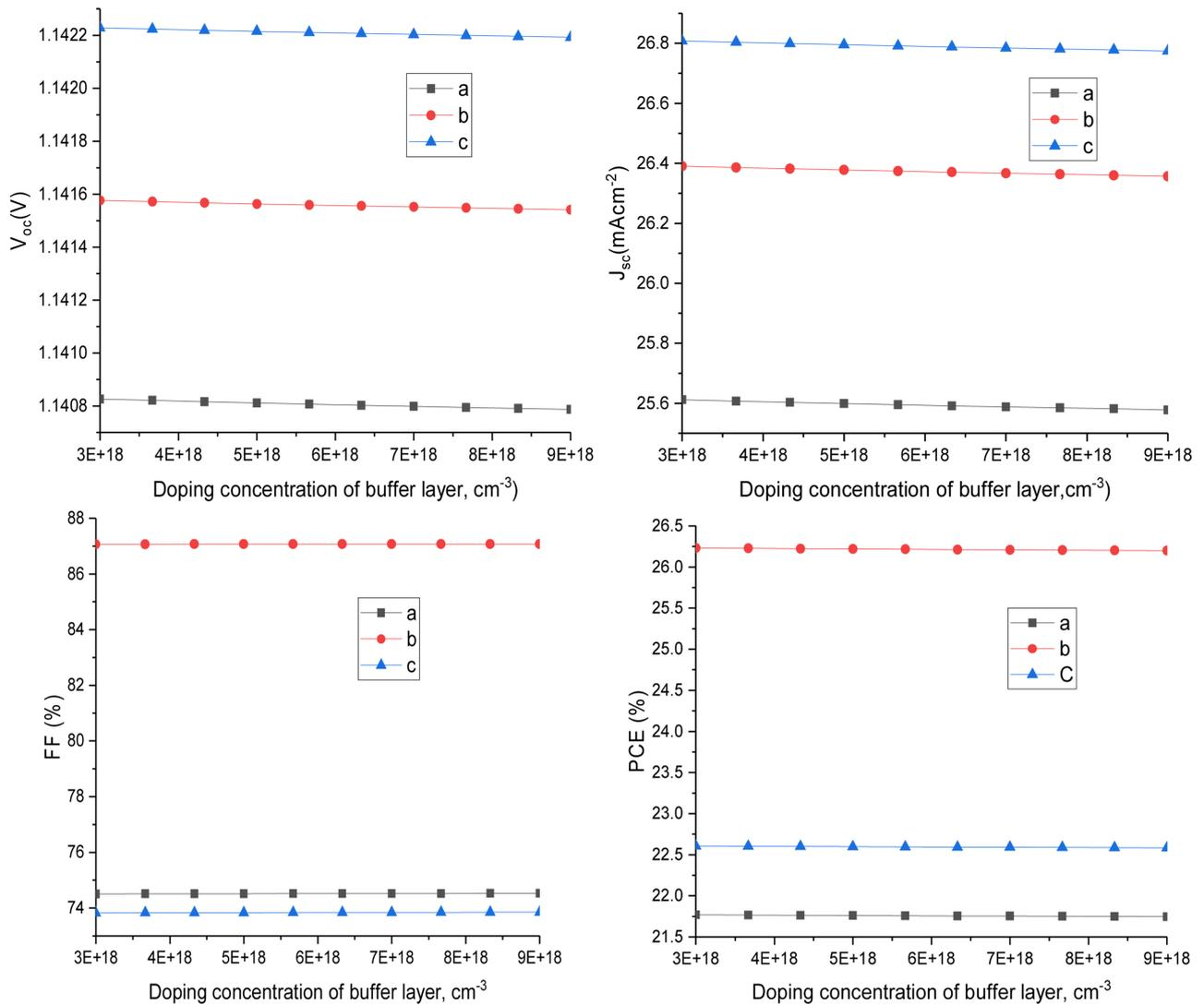
**Figure 5.** The impact of buffer layer doping concentration ( $a = 0.6 \mu\text{m}$ ,  $c = 1 \mu\text{m}$ ,  $b = 0.8$ ).
