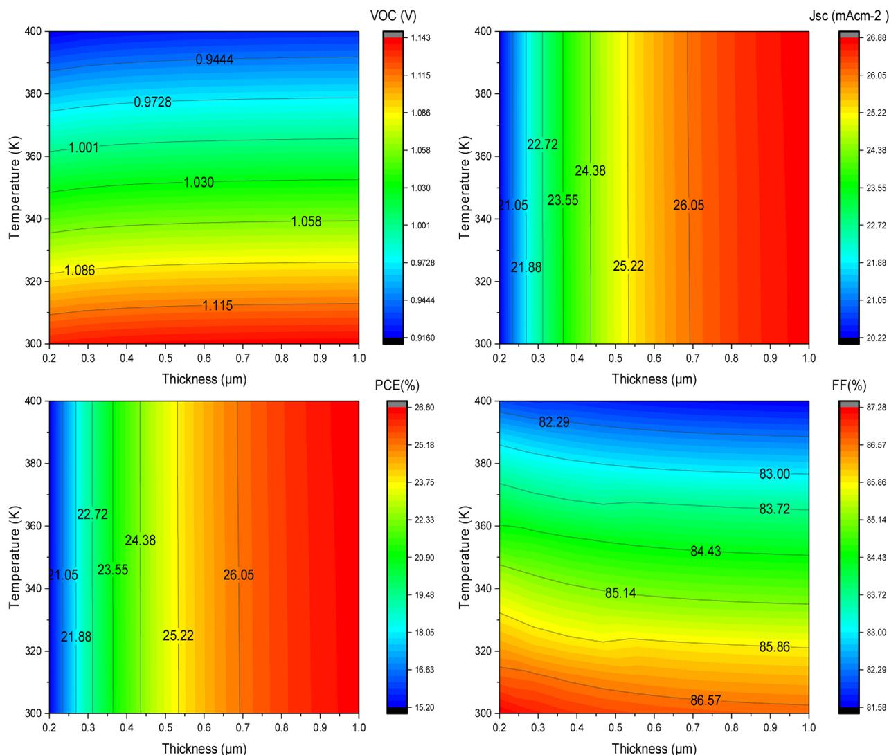
**Figure 6.** Contour graph the variation of CSSnCl<sub>3</sub> cell performance with temperature and the thickness of the absorber layer.
