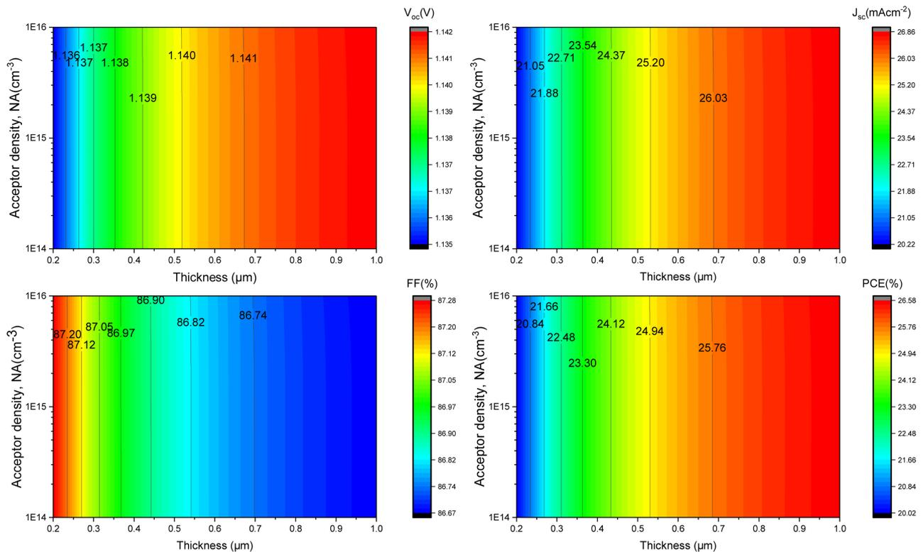
**Figure 7.** The effect of the thickness and acceptor density of  $\text{CsSnCl}_3$  on the solar cell electrical properties.
