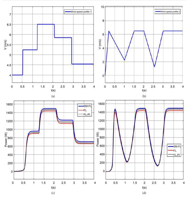
Figure 7. The powers obtained with the two wind profiles and their zoom.
