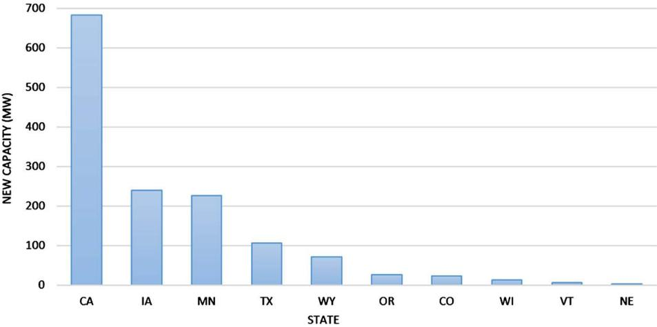
Figure 4. Total new wind energy capacity in the 1990s by state (Top 10 states in the 1990s).
