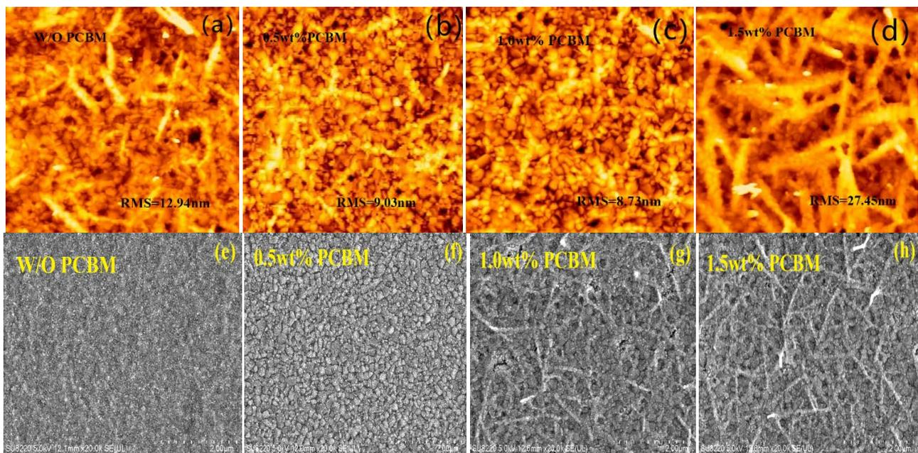
**Figure 3.** AFM images of MAPbI<sub>3</sub> perovskite thin films with different fabrication approaches. (a) W/O PCBM; (b) 0.5 wt% PCBM; (c) 1.0 wt% PCBM; (d) 1.5 wt% PCBM; (e)-(h) Top-view SEM morphology characterization of perovskite MAPbI<sub>3</sub> films without and with PCBM 0.5 wt%, 1.0 wt%, and 1.5 wt%.
