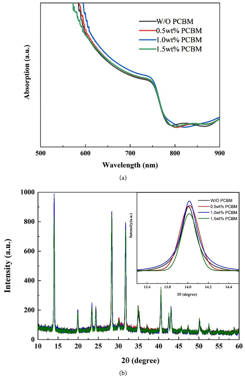
**Figure 2.** (a) UV-Vis absorption spectrum of the perovskite films with different doses of PCBM; (b) XRD patterns of pristine perovskite and PCBM-perovskite films.
