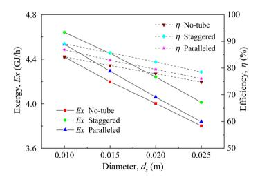
**Figure 8.** Effects of particle diameter on exergy and waste heat utilization efficiency.
