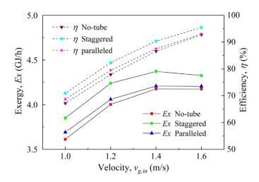
**Figure 11.** Exergy and waste heat utilization efficiency in device with different pipe arrangement.
