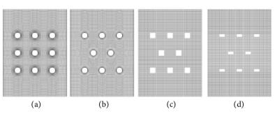
**Figure 1.** Waste heat recovery device with different internal components. (a) Paralleled; (b) Staggered; (c) Quadrate; (d) Rectangle.
