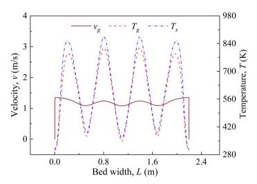
**Figure 3.** Temperature and velocity changes in horizontal directions of paralleled device (y = 1.25 m).
