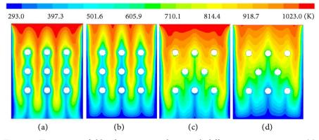
**Figure 2.** Temperature field in heat recovery device with different pipe arrangement. (a) Air temperature; (b) Particle temperature; (c) Air temperature; (d) Particle temperature.
