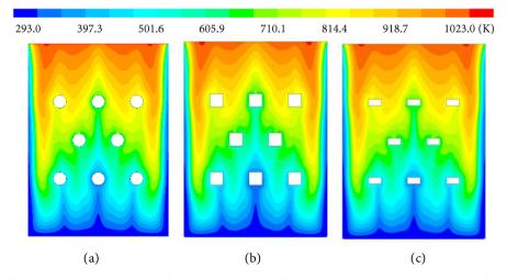
**Figure 13.** Temperature fields in device with different shapes of component. (a) Circle component; (b) Quadrate component; (c) Rectangle component.
