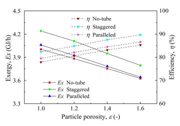
**Figure 10.** Exergy and waste heat utilization efficiency with different particle porosity.
