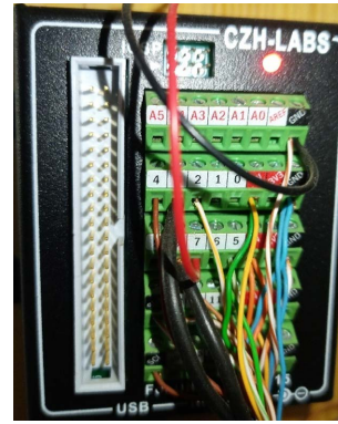
Figure 3. Arduino 1 board in aluminium housing with screw terminal bypass module.
