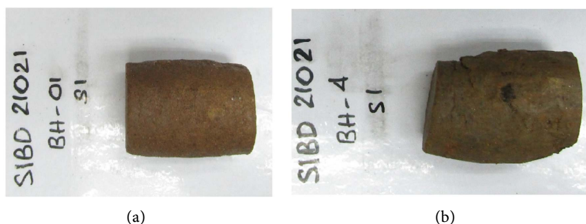
Figure 2. Failure nature—(a) Bulging and (b) Shear in Triaxial Consolidated Undrained test.
