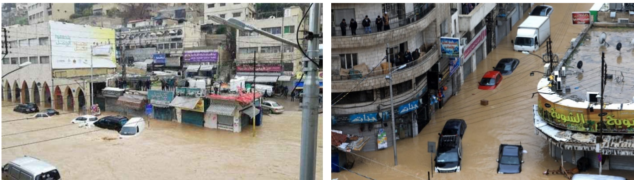
Figure 4. Amman flooding events in 2015 & 2023 showing parts of the old city, where the designed drainage system has become undersized due to increasing urbanization and increasing rain intensities.
