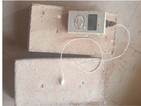
Figure 10. Thermal testing of cement mortar samples.
