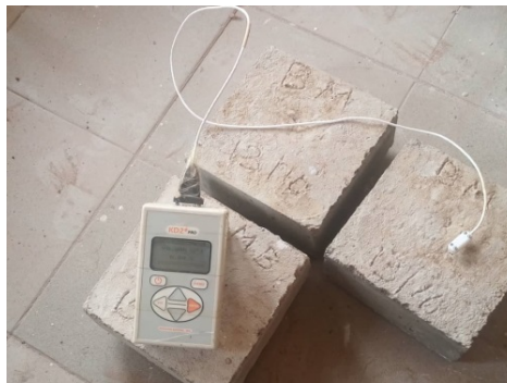
Figure 11. Thermal testing of concrete samples.
