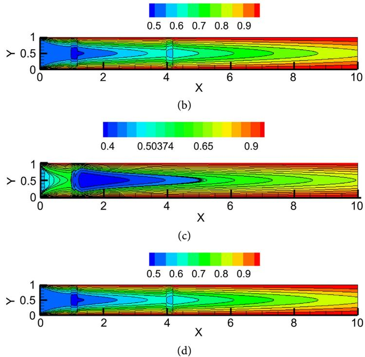
**Figure 2.** The normalized temperature profile plotted for  $Re = 100$  using statistical technique (a) for single strainer, (b) for a double strainers and quantum technique (FDM) for (c) for a single strainer, (d) for double strainers.
