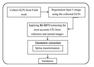
Figure 1. Flowchart of the geometric correction model.
