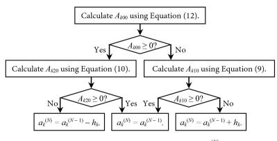
**Figure 6.** The constant iteration algorithm for calculation  $a_k^{(N)}$ .
