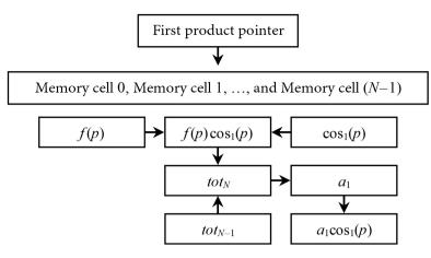
**Figure 2.** The block diagram of the memory cells and calculation process of the direct calculation algorithm for calculating  $a_i^* \cos(\omega t)$ .
