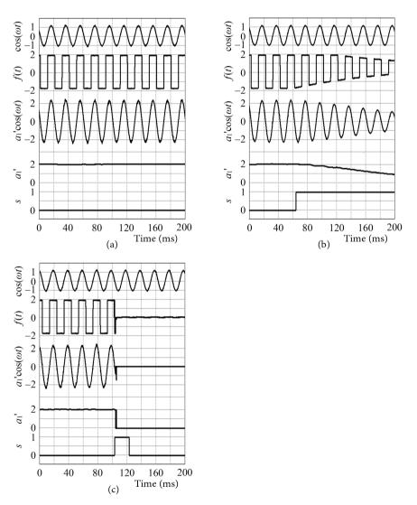
**Figure 13.** (a)-(c) The experimental results of the biproportional construction algorithm for calculating  $a_1^* \cos(\omega t)$  with no change, a slow decrease, and a step decrease, respectively, in f(t).
