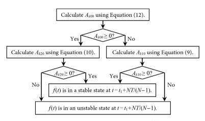
**Figure 10.** The algorithm for determining the state of f(t) at the sampling time  $t = t_1 + NT/(N-1)$  based on the optimal iteration algorithm.
