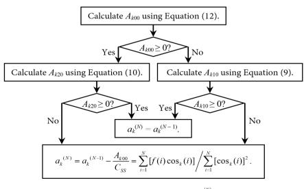
**Figure 8.** The optimal iteration algorithm for calculating  $a_k^{(N)}$ .
