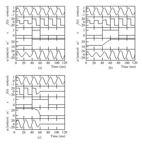
**Figure 12.** (a)-(c) The simulation results of the biproportional construction algorithm for calculating  $a_i^* \cos(\omega t)$  with a step increase, a linear increase, and an exponential decrease, respectively, in f(t).
