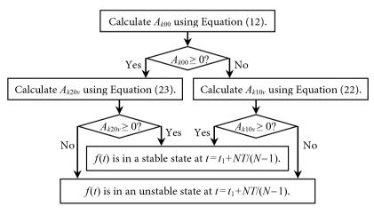
**Figure 11.** The algorithm for determining the state of f(t) at the sampling time  $t = t_1 + NT/(N-1)$  based on the variable iteration step.
