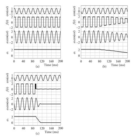
**Figure 5.** (a)-(c) The experimental results of the direct calculation algorithm for calculating  $a_1^* \cos(\omega t)$  with no change, a slow decrease, and a step decrease, respectively, in f(t).
