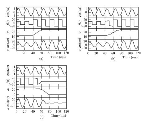
**Figure 7.** (a)-(c) The simulation results of the constant iteration algorithm for calculating  $a_1^* \cos(\omega t)$  with a step increase, a linear increase, and an exponential decrease, respectively, in f(t).
