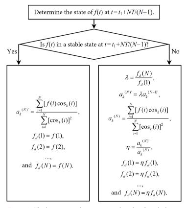
**Figure 9.** The biproportional construction algorithm for calculating  $a_k^{(N)'}$ .
