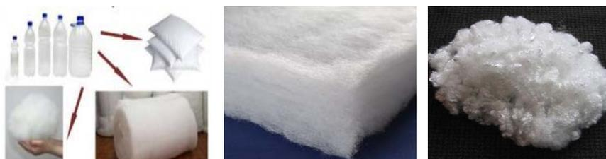
**Figure 1.** Heat-insulating nonwovens.
