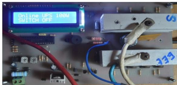
**Figure 10.** DSP control UPS system at power mode.
