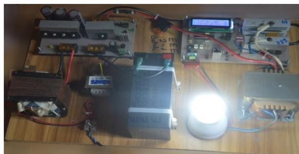
**Figure 11.** Completed UPS system with physical output.
