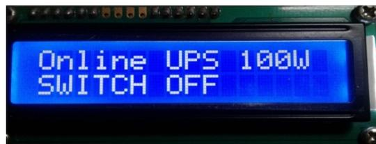
Figure 5. Result on LCD LM016L at off stage.
