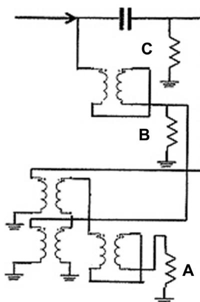
**Figure 7.** One-way signal converting to three-phase (A, B and C) signals.
