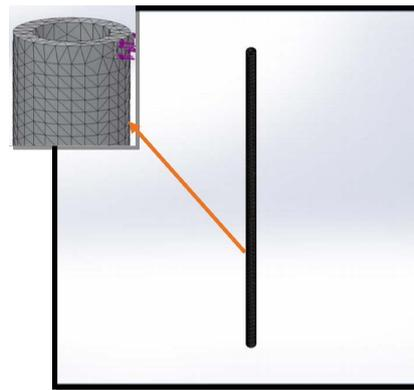
Figure 5. Meshing of the spacer.
