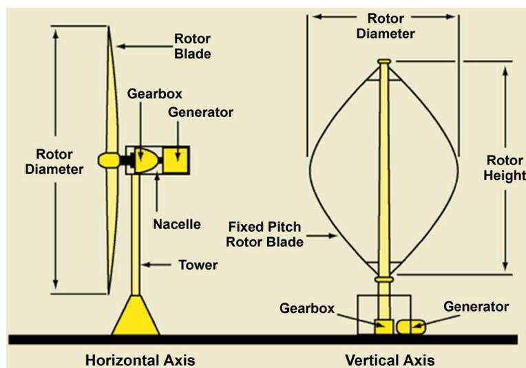
**Figure 1.** Horizontal & Vertical axis wind turbine [7].
