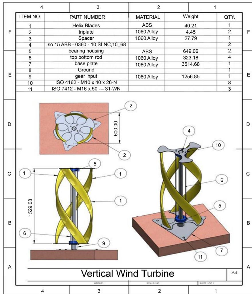
**Figure 3.** CAD design with basic dimension and Bill of Material from solidworks.
