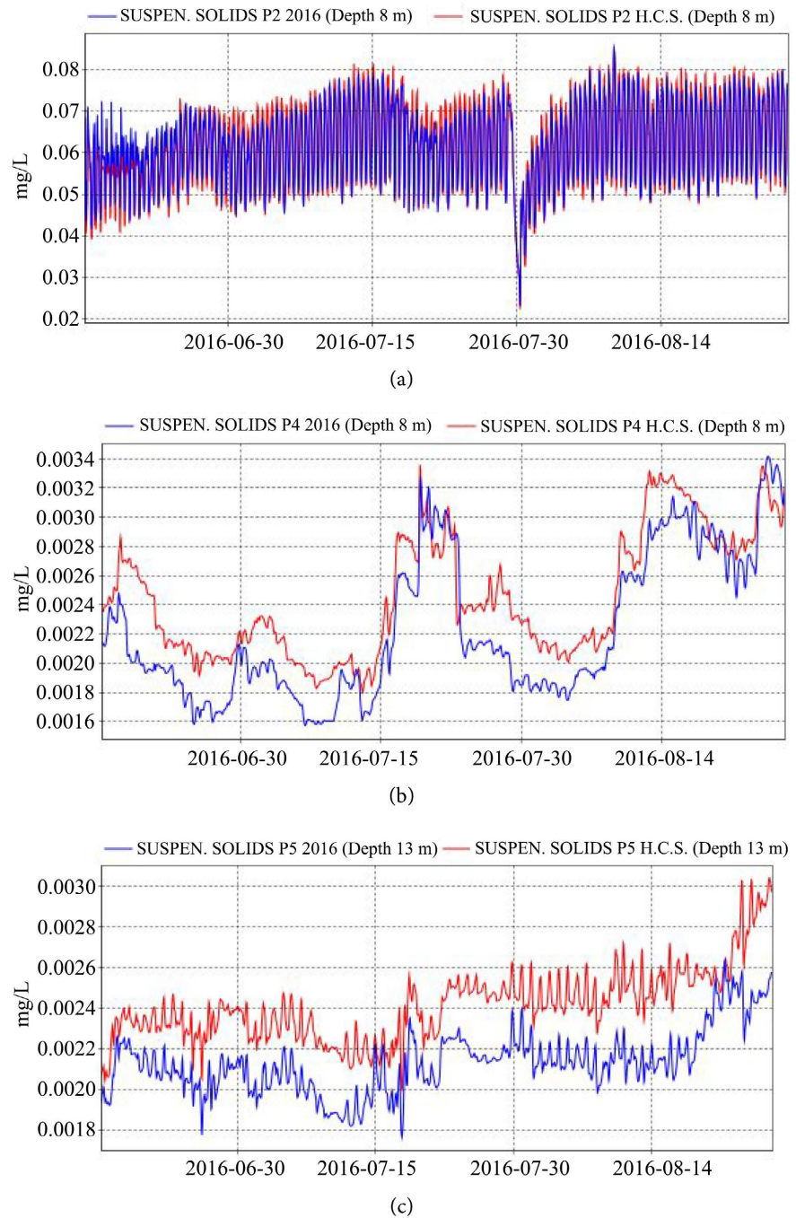
Figure 16. Comparison of suspended particulate matter concentration during the warmest period of the simulations from 15 June to 27 August, as derived with AEM3ED software for the year 2016 and for the year of the hypothetical climate scenario (H.C.S. for short), (a) At point P2 in the CHALKIS area in the 8 m bottom layer, (b) At point P4 in the AMARINTHOS area in the 8 m bottom layer and (c) At point P5 in the ALIVERI area in the 13 m bottom layer.
