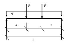
Figure 2. Four-point bending schematics.
