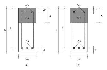
Figure 3. Cross-section of rectangular beam.
