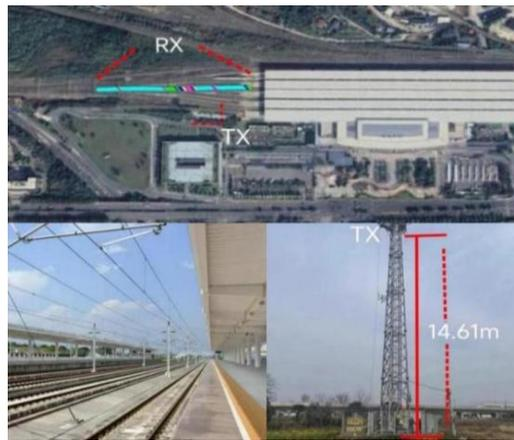
**Figure 6.** The GPS location and the antennas channel sounder.
