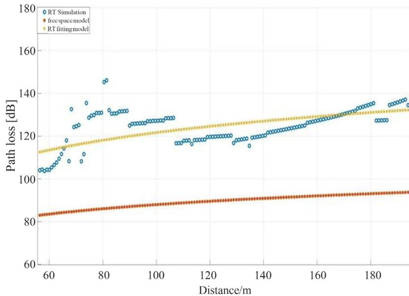
**Figure 7.** Wireless channel path loss analysis.
