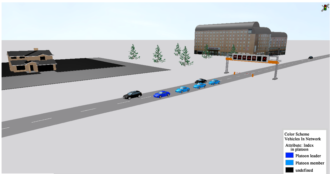
Figure 13. Execution screen of VISSIM simulation for toll collection for platoons in the ETC method.
