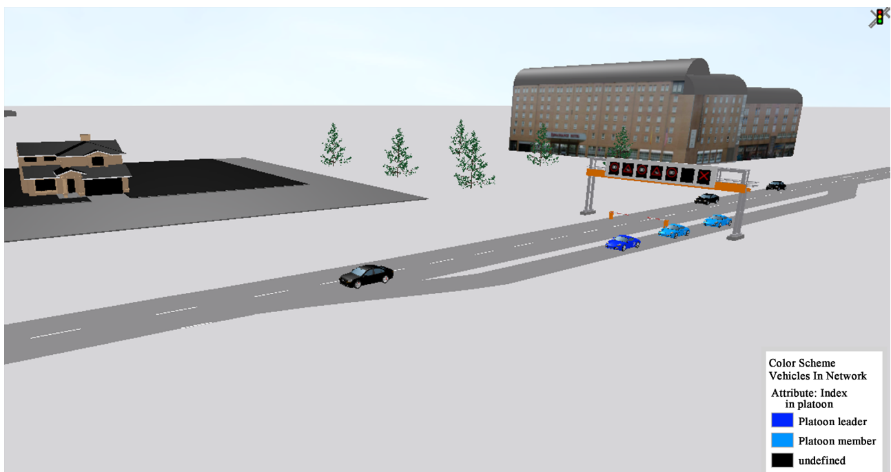
Figure 14. Execution screen of VISSIM simulation for toll collection of platoons in the ETC and freeway road lane method.
