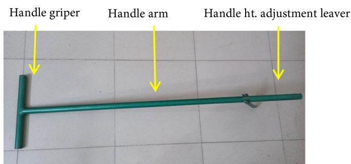
Figure 10. Photographic view of the handle of the weeder.
