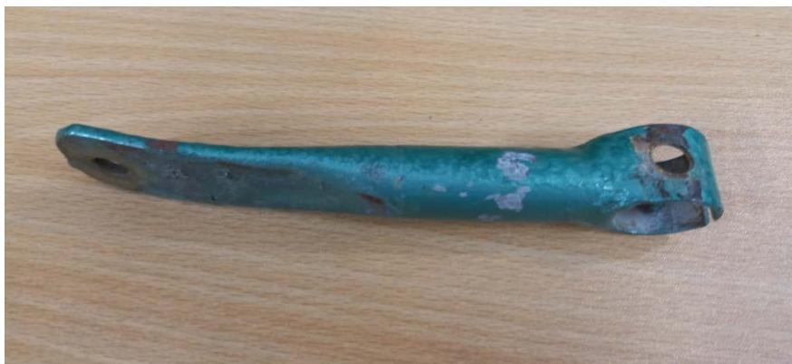
Figure 12. Photographic view of the rotor holder of the weeder.
