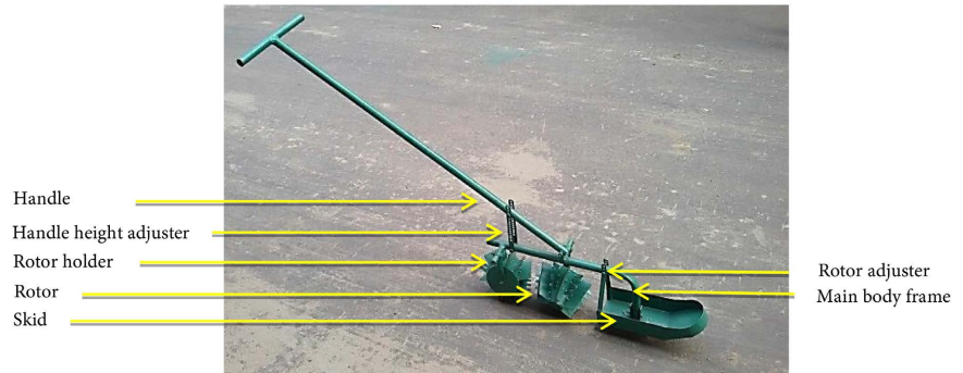
Figure 1. Photographic view of the conical weeder.
