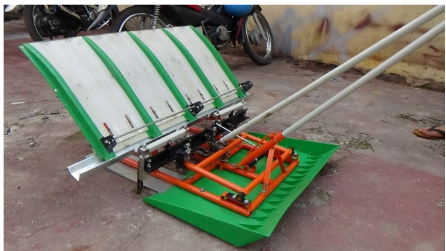
Figure 1. Field operation of the BRRRI developed manual rice transplanter.
