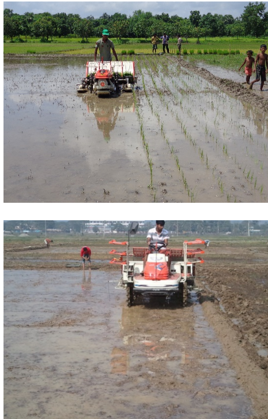
Figure 2. Field operation of the walk behind type and riding type rice transplanter.
