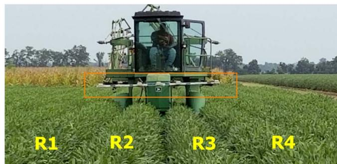
**Figure 2.** Data collection (August 8, 2019) of soybeans with mobile plant height and plant canopy temperature system—enclosed in orange square. R1, R2, R3 and R4—rows 1 - 4 of transect. Vehicle is traveling in the north to south direction.
