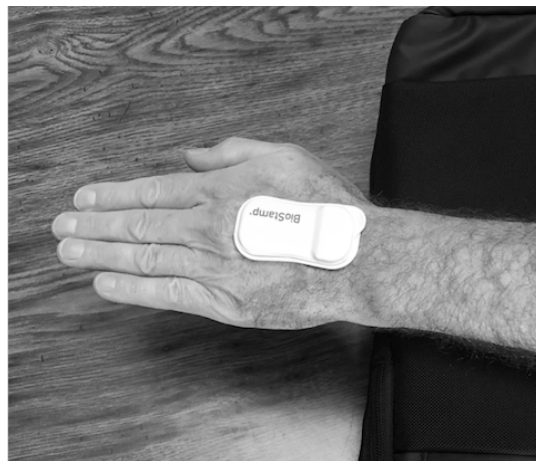
Figure 1. The BioStamp nPoint mounted by adhesive medium to the dorsum of the hand.
